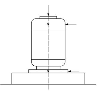
NOTE Measurements to be made at the bearing housing or, if not accessible, then at positions as close as possible to the bearing housings which provide adequate sensitivity to the machine dynamic forces.
