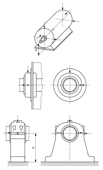
NOTE Measurements to be made at the bearing housing or, if not accessible, then at positions as close as possible to the bearing housings which provide adequate sensitivity to the machine dynamic forces.
