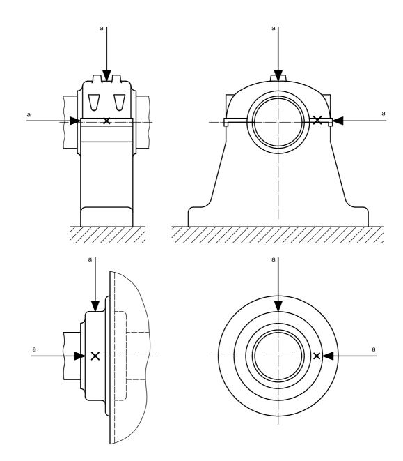
NOTE The evaluation criteria in this part of ISO 10816 are applicable to radial vibration on all main bearings and to axial vibration on thrust bearings.
