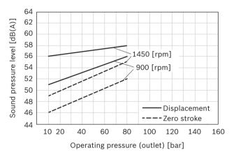
16 **PV7 Series 1X** | Adjustable vane pump, pilot-operated Characteristic curves for frame size 25
