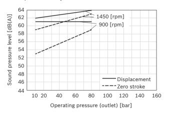
18 **PV7 Series 1X** | Adjustable vane pump, pilot-operated Characteristic curves for frame size 63
